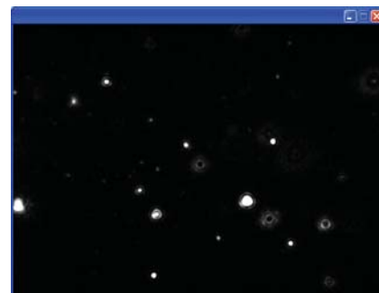
LM20 view of Cerium oxide particles dispersed in organic solvent. The image clearly shows a range of particle sizes with the dimmest particles representing a population of small particles.
